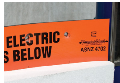
TransNet Cable Cover undergoing a penetration test
